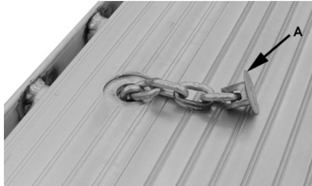
Figure 7-1 Trailer Equipped With Chain Tie Downs
